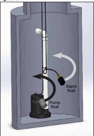
**Perform final testing on system** by lifting pump and alarm float. When pump float is lifted, the pump will turn on. When alarm float is lifted, the alarm horn will sound and alarm light will illuminate.
