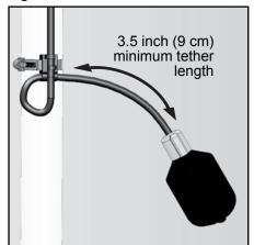
Install alarm float and pump float. (Mounting Clamp detail)
